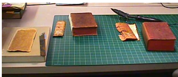
Stages of leather spine repair: 1. Paring the new leather, 2. Old spine removed from book, 3. Finished book with new leather spine.
